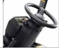
The FGC15N-FGC33N series comes standard with the Integrated Presence System (IPS), which is designed to disengage all powered travel and some hydraulic functionality when the operator leaves the normal operating position. Additionally, warning alarms sound and indicators are shown on the display panel, informing the operator and surrounding personnel that the system is engaged.
