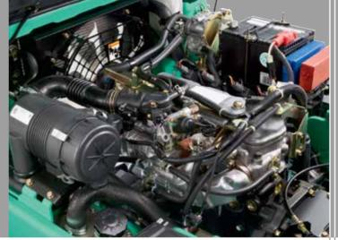
Cool And Quiet: The forklift's fan and radiator system is equipped with a horizontal cross flow cooling system to help keep the engine cool and functioning at peak performance. The corrugated design provides optimal heat exchange, while the aluminum core helps to prevent corrosion. The direct drive fan also reduces noise and necessary maintenance, benefiting your operators and your business.
